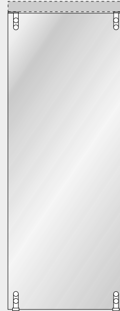
HSW-GP Fully glazed with single-point fixings
